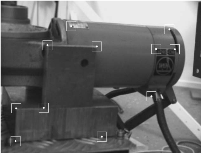
Fig. 5. Image of the compliant environment, with some of the features used for measurement of the deflection of the compliant tool in a single degree of freedom
