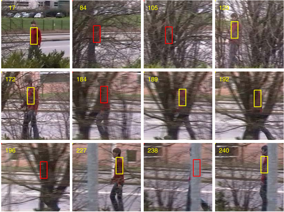
Fig. 2. Tracking under severe occlusions. The color-based tracker is initialized on the top of the walking person. The succession of occlusions caused by foreground trees is successfully handled thanks to the explicit modeling of visibility changes. The box corresponds to the MC approximation of the posterior state expectation. Its color is changed from yellow to red when the posterior visibility probability drops below 0.5.
