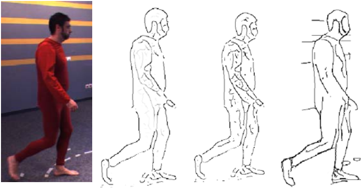
Fig. 5. (a) Original color image. (b) Standard Canny filter. (c) Color Canny filter detects the contours partially better but there still exists plenty of distracting edges. (d) Anisotropic Gaussian color filter reveals the full boundary edges.
