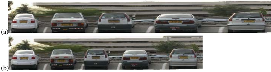
Fig. 8. Mosaicing from a translating camera with motion parallax. (a) Using regular 2D parametric image alignment. Distortions occur when image motion alternates between far and near objects. (b) Using predictive alignment all cars are properly scaled.
