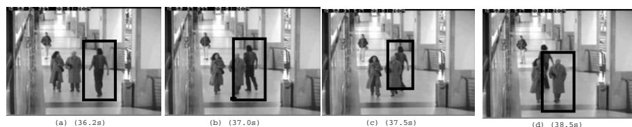
Fig. 11. Weakness of the method. The tracker fails and changes of target during the sequence because the new target has a higher classifier score than the initial one.
