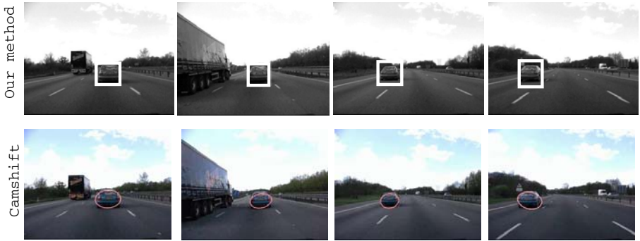
Fig. 8. Example of vehicle tracking (The video sequence comes from PETS database: Performance Evaluation of Tracking and Surveillance). Upper images show results obtained for the tracker and lower images show results obtained for the CAMSHIFT Tracker.
