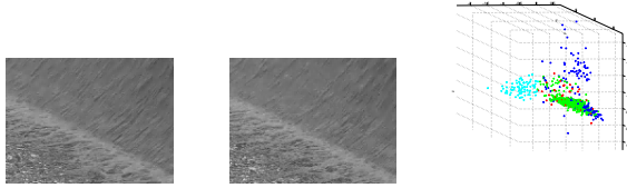
Fig. 2. Left and Middle: two images from a 300-frame sequence of water flowing down a dam. Right: the 3-D projection of the data points with N = 300 and l = 5 . Different colors identify different groups segmented using GPCA as described later.
